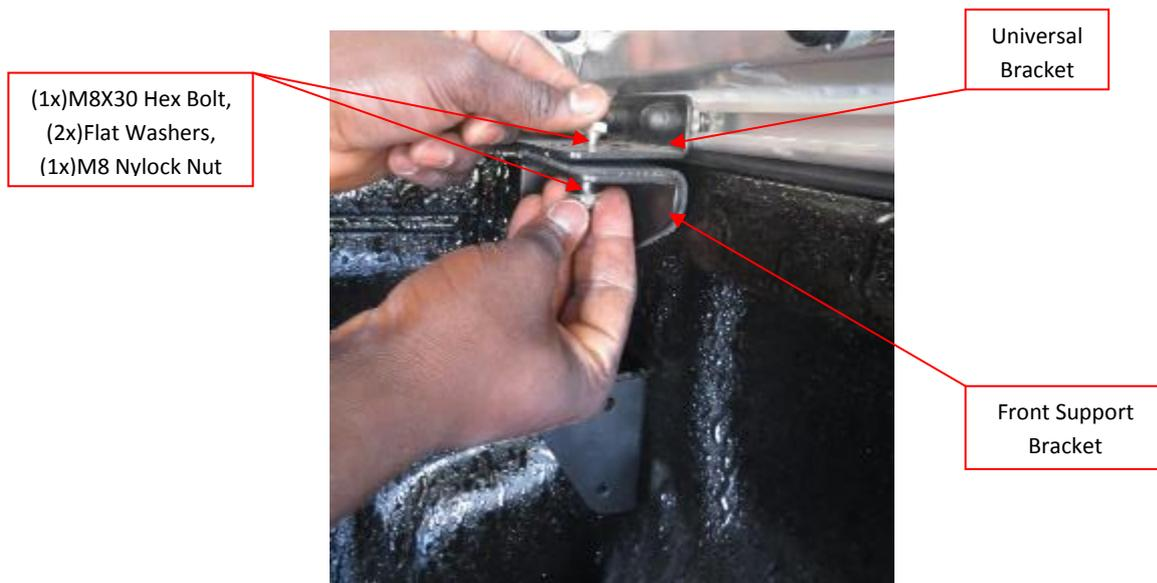
Figure 19: Inserting Bolt for Universal-Front Right Support Bracket
