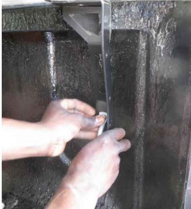
Figure 8: Aligning the Rear Support Bracket
