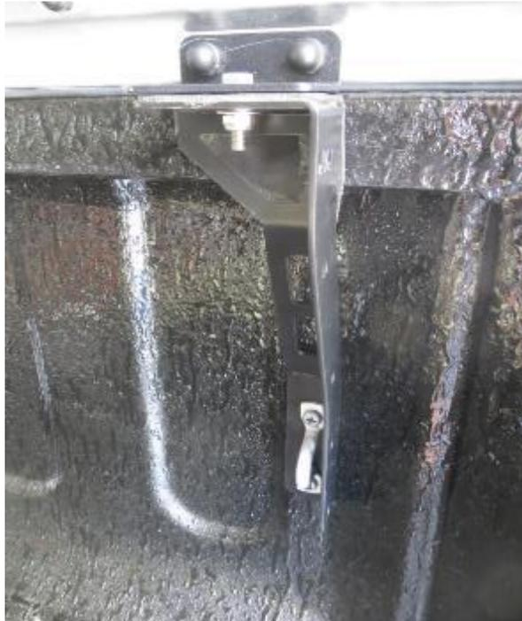
Figure 18: Rear-Right Support Bracket Installed
