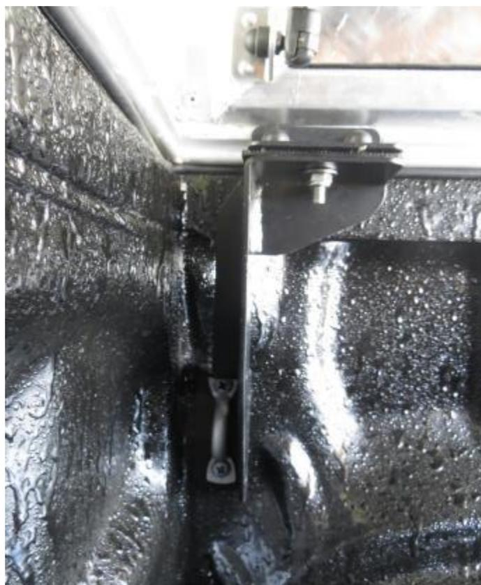
Figure 21: Front-Right Support Bracket Installed
